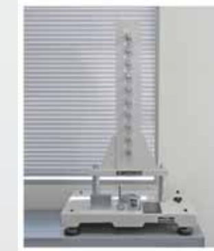
Loading weight: 1,000 g Drop height: 50 cm
