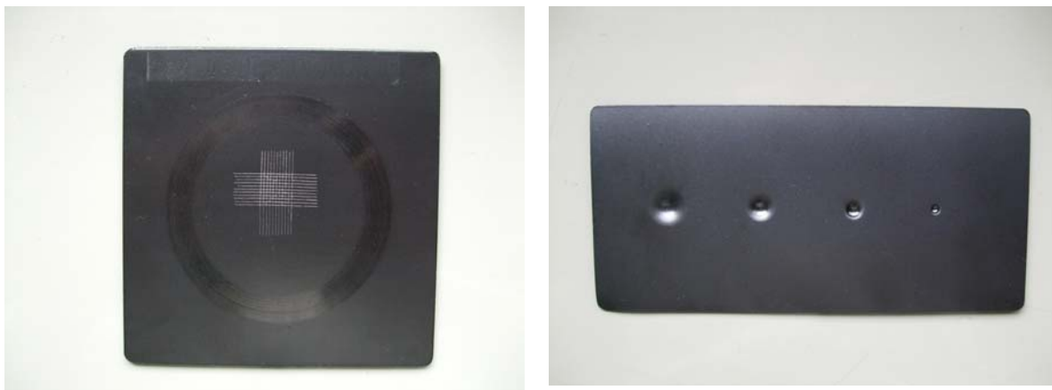
Nanotect-A after a 500,000r of abrasion test (left) and a 1.6mm \phi /1kg/50cm Du-Pont test (right)
