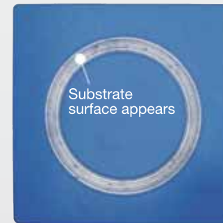
Typical organic polymer coating (4,000 cycles)
