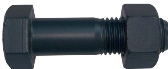
Nanotect-C after 3000h of salt spray test
